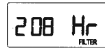
Image shows the filter counter at 208 hours. The filter icon illuminates in the primary display at 500 hours.
