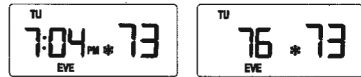
Image shows room temperature of 76° and A/C set point of 73° as the display alternates every 3 seconds.
